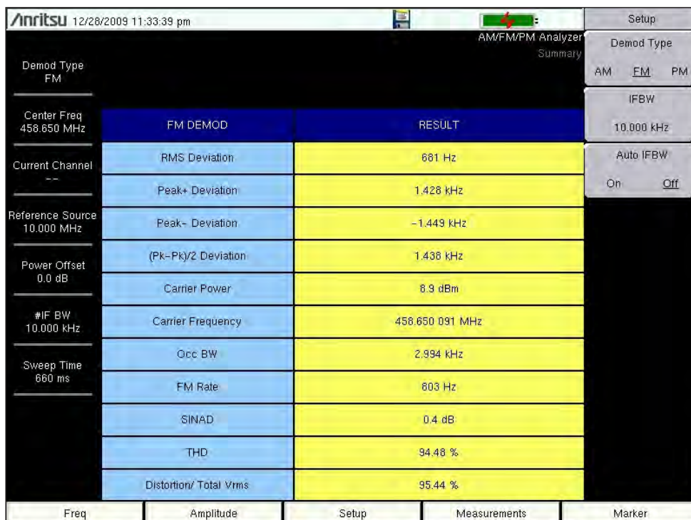
Figure 9. The FM Demod mode MMS display screen data of the Kenwood NXD-300 NXDN radio in the ultra-narrowband 6.25 kHz mode
