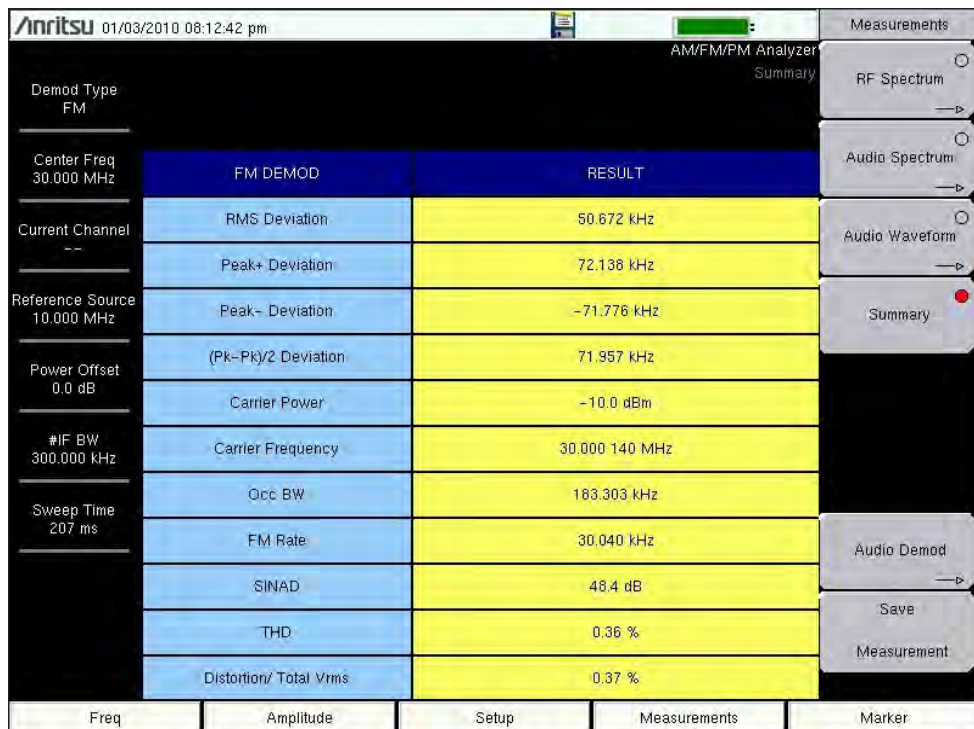
Figure 4. The MMS summary display screen for the 30 MHz signal with F_m = 30 kHz sinewave modulation and F_{dev} = 72.144 kHz.
