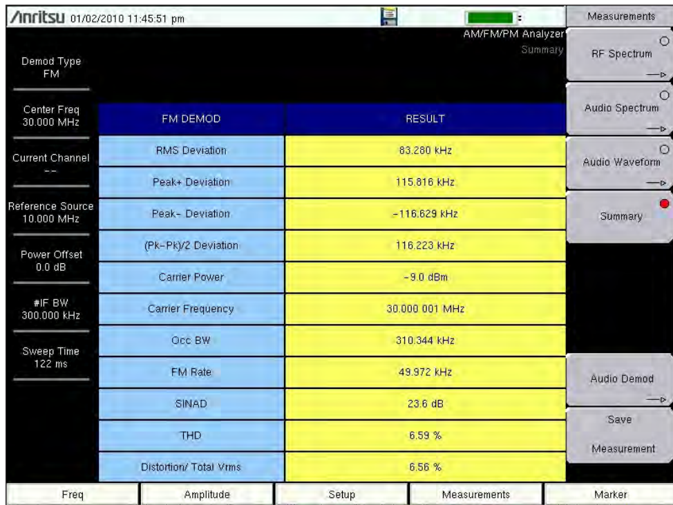
Figure 3. The MMS summary display screen for the 30 MHz signal in Figure 2 with F_m = 50.0 kHz and F_{dev} = 120.24 kHz.
