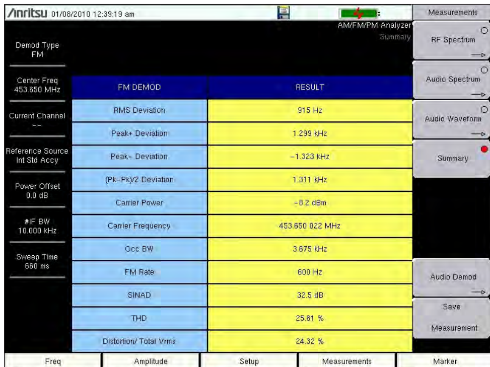
Figure 11. The FM Demod mode MMS display screen data of the Kenwood NX-300 NXDN radio in the 6.25 kHz ultra-narrowband (UNB) deviation alignment mode.
