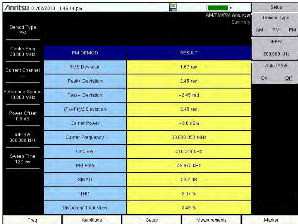
Figure 12. MMS display screen for PM demod measurement of the 30 MHz signal shown in Figure 2 with 50 kHz sinewave FM modulation and 120.24 kHz deviation.
