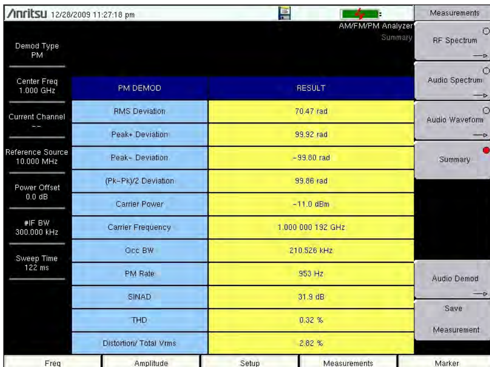
Figure 6. The PM Demod mode MMS display screen data for the Figure 5 PM signal with 1 kHz modulation and 100 rads phase deviation.
